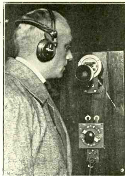
THE new liner Berlin is the first ship to be equipped with radio telephone booths for the use of passengers. Photo shows a passenger, Dietrich Berbeg, talking over phone in booth. It is connected with the ship's radio room, where all the sending and receiving apparatus is located, and is connected much like a regular telephone switchboard. With this radio telephone passengers can talk to other ships within a few hundred miles. (Fotograms.)
